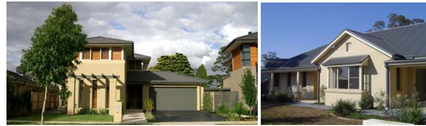
Single storey elements help to reduce the bulk of predominantly two storey dwellings (left) while bay windows and verandahs introduce interest to facades (right)
