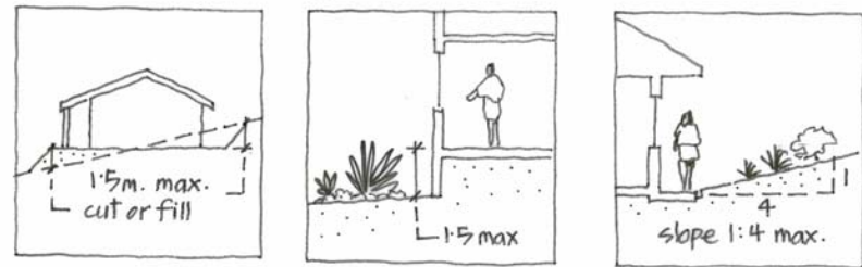
Minimise cut and fill, exposed areas and the slope of embankments
